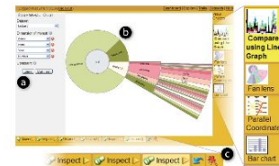
Figure 1. Behavior-driven visualization recommendation has been integrated into our lab's visualization system. Users can (a) issue queries and (b) interact with visualizations to analyze data. When a new recommendation is provided due to a user's behavior, he/she is notified via (c) a magic wand icon in the history panel and (d) a flashing segment on the recommendation sidebar. Users can accept the recommendation with a single click, or ignore it to continue uninterrupted.
